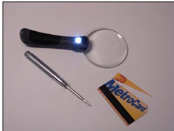
A lighted magnifying glass, screwdriver, and a crevice tool made from a NYC Metro Card are all very useful for inspecting. Photo by J. Gangloff-Kaufmann
